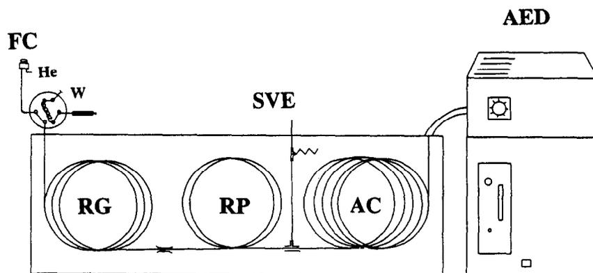
Fig. 2. Instrument configuration of large-volume injection GC-AED. AC = Analytical column; FC = flow controller; RG = retention gap; RP = retaining precolumn; SVE = solvent vapour exit; W = waste.
